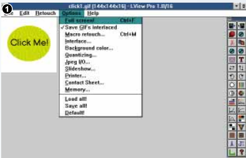
Fig 1 When you've loaded the picture into Lview, select the Options menu and then choose Background colour. If you don't have a copy of Lview, you can download it from ftp.demon.co.uk, in the simtell/win3/graphics directory
